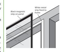
HELPFUL HINTS - For larger windows (1200mm x 1200mm or bigger) we strongly recommend placing a couple of screws under the glazing panel to support the sheet. This will remove the risk of the sheet from slipping down and becoming detached.
